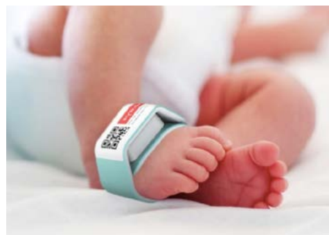
Figure 1. Boppli™ device to monitor the blood pressure of infants in critical care.
